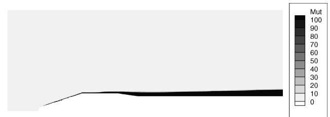
Fig. 6 Turbulent viscosity contours for the case with Liou's second-order scheme and Spalart and Allmaras model, M_\infty = 0.90 and Re = 20 \times 10^6 .
